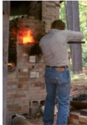
Kurt Heinzman stokes a shovel-full of hardwood charcoal onto the unglazed wares during the "yohen" treatment of chamber four at the 2002 workshop.
